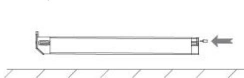
3. Find a fuse in the plastic transparent bag and insert a fuse into the battery (Labeling on top). Then put the battery back into the baseboard and lock the battery.
