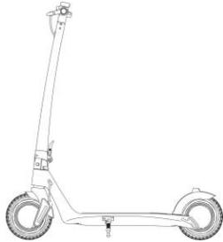
3. Insert the exposed cable into the front bar. Then insert the handle bar into the front bar as well. Use the tool and screws to bolt the handlebar to the front bar.
