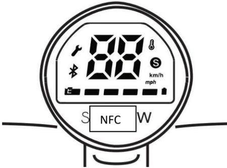
For Android, open the SoFlow App, connect your scooter, and then touch NFC to lock or unlock it.
